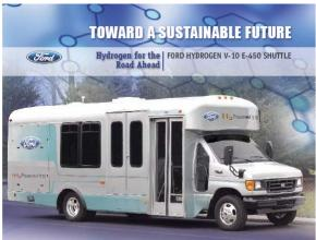
provide LYNX four hydrogen-powered buses. The vehicles will seat nine passengers, including one wheelchair securement position.
