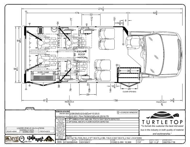
The proposed procurement will be for fifteen (15) Turtle Top "Odyssey" models (pictured), to be built on Ford chassis with three varying seating capacities on each vehicle (using foldaway seating) of:
